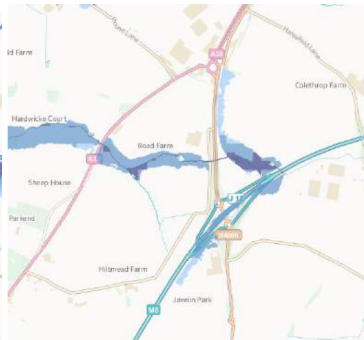
Figure 10. Extent of Fluvial Flooding
