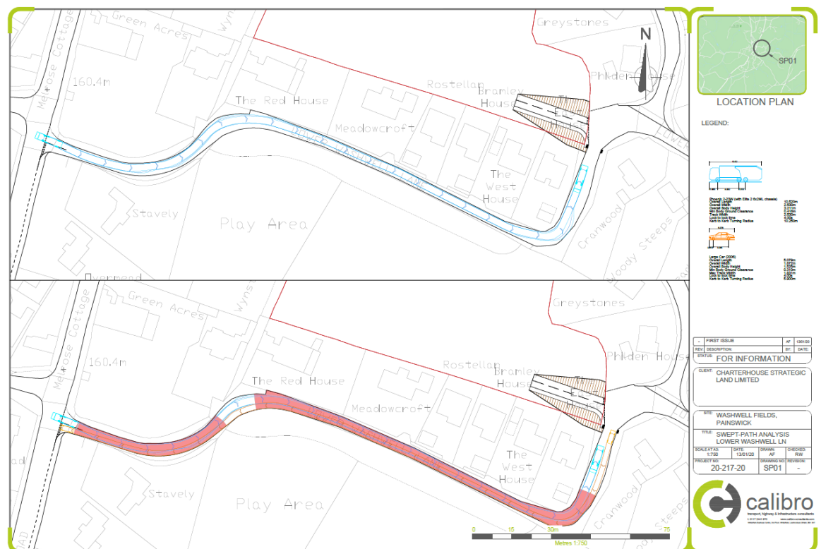
Figure 8 - Refuse Vehicle Swept-Path Analysis
