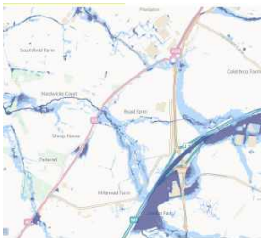
Figure 9. Extent of Surface Water Flooding
