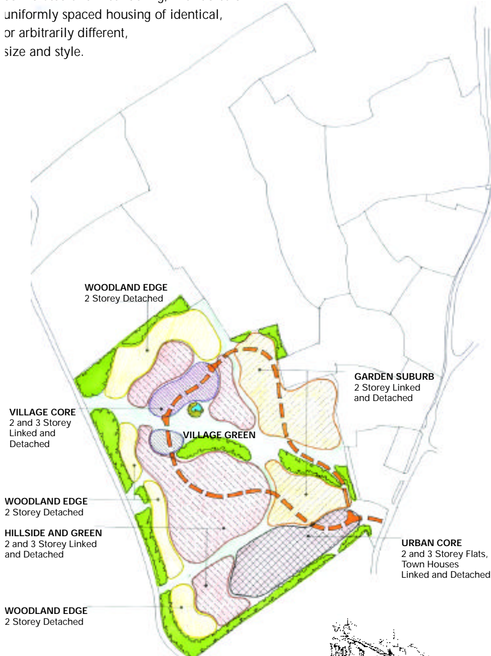
Concept plan for a new housing site showing zones of different character
