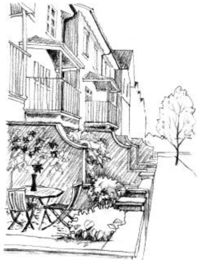
In this housing scheme in Bristol, screen walls form a feature of the design and provide a measure of privacy
